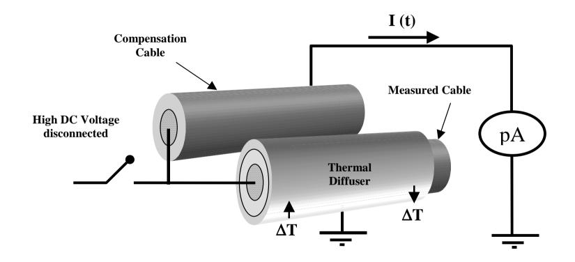
Compensation of cable polarization and conduction current
