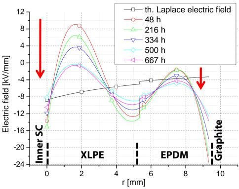
Field enhancement at electrodes indicates heterocharges
